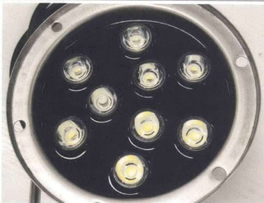
Photo 5: Test result after IP6X and IPX8 test
